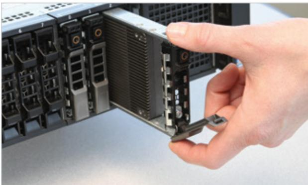
**An Easy Hot Swap:** The P420m 2.5-inch form factor can be easily inserted/removed from the front of a server without removing the server from the rack or turning off power. This dramatically improves serviceability and lowers total cost of ownership.
